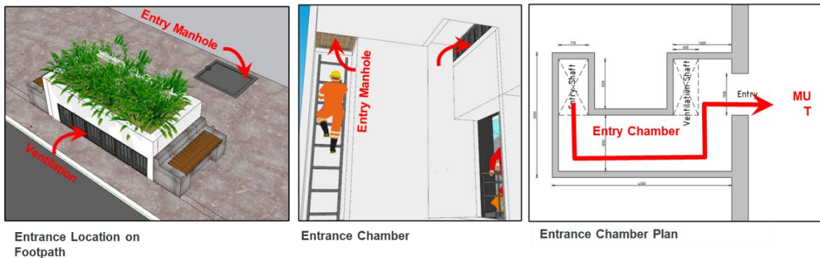
Figure 2.7 Proposed Multi Utility Tunnel Entrance Section
