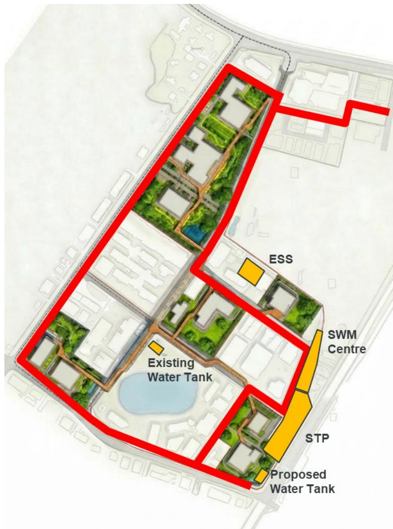
Figure 2.8 Proposed Multi Utility Tunnel (Peripheral) Network
